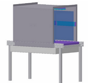
UVC conveyer tunnel
