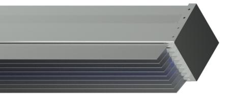
Cerberus Wall is open type lamp for wall installations, designed for upper room free-flowing-air disinfection. UV-C irradiation is emitted above the horizontal plane, which forms the bottom of the upper room volume, through upwards focussed louvres. To prevent damage to skin and retina recommended installation height is no less then 2,4m off the ground level
