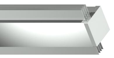
Cerberus® Ceiling UV-C Lamp is an open type device for ceiling installations, designed for air re-circulation and upper room free-flowing air disinfection. Dual function of sideways irradiation via open louvers for the upper room disinfection and active inflow of air from below area with an immediate disinfection of passing air
